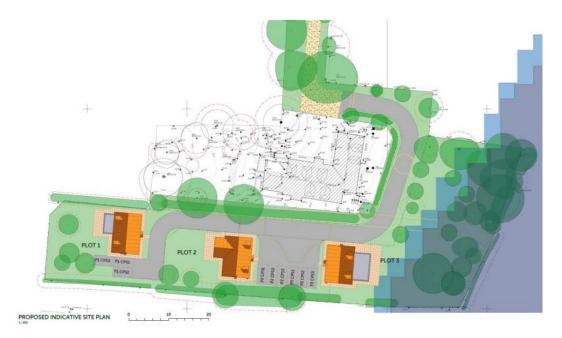
Figure 3 - Site plan overlain with flood zones
